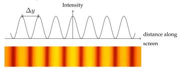
If the slit separation is a and the observation point is a distance D away (see diagram), then the width of the fringes  $\Delta y$  is given by
