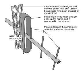
If there is more than one such aerial, the one for TV is the one with the shortest rods. The rods may be vertical or horizontal. The aerial points towards the TV station. Estimate the length of the rods, top to bottom (look for something like chimney bricks whose size you know to guess the length).
