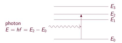
An electron jumps into a higher-energy excited state, and the photon has ceased to exist.
