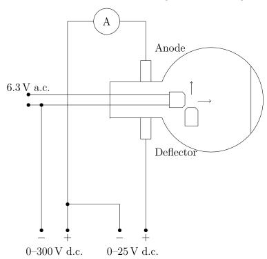
Once all the connexions have been made, make sure the anode voltage is zero (the control knob should be turned anticlockwise as far as possible), before turning on the power supply to the metal filament.
