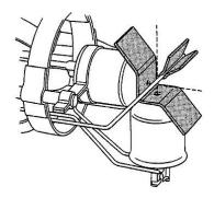
Just outside each gun muzzle there is a pair of plates for deflecting the beam by an electric field. One plate of each pair is attached directly to the gun muzzle which supports it. The other plate of each pair is connected inside the tube to the second side terminal on the tube. If the beam fails to make a clear spot then try a small potential difference to the deflecting plates.
