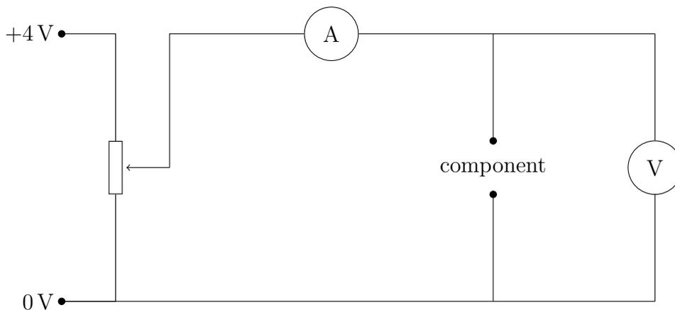
1. Using the variable resistor (and if necessary the voltage setting on the power supply), measure the current through the ohmic conductor for voltages between 0.00 V and 0.60 V, in 0.10 V steps.
