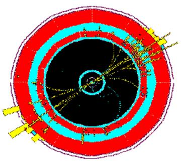
The picture above is a reconstruction of a collision in ALEPH. The e<sup>+</sup> and e<sup>-</sup> annihilated and a quark and antiquark were created, each evolving into a jet of several other particles. Particles of opposite charge are bent in opposite directions in the magnetic field. The different particles interact in different ways in the outer layers of the detector allowing them to be identified.
