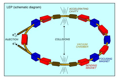
The same features seen in the television set are found in the LEP accelerator at CERN but on a larger scale (27km in circumference, over 4000 magnets). LEP accelerates electrons and positrons to 50GeV before they collide.
