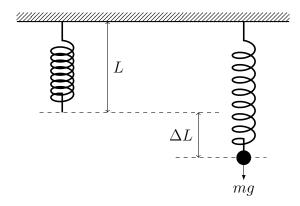
The way in which the length of a spring depends on the force on it was first investigated in the seventeenth century by Robert Hooke. He discovered that the extension of a spring from its natural length is directly proportional to the force applied to it and this is known as Hooke's law. Mathematically,
