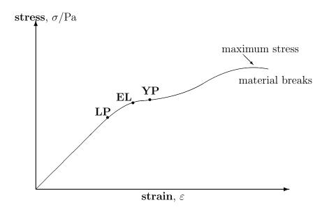
The extension of a typical ductile material in tension is shown on the graph above. As the material is extended, the stress needed on the object is plotted out.
