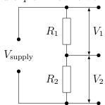
A potential or voltage divider provides a convenient way of getting a variable voltage from a fixed voltage supply. The voltages appearing across the resistors  $R_1$  and  $R_2$  are in the ratio of their resistances, i.e.  $V_1/V_2 = R_1/R_2$ .
