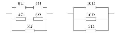
The final combined resistance  $R_f$  can now be calculated from the resistances of the three parallel branches:
