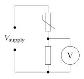
The reading on the voltmeter can be calibrated to give an indication of the temperature at the thermistor. Most thermistors are negative temperature coefficient (NTC), in which the resistance decreases with increasing temperature; therefore the voltage across the bottom resistor will increase with increasing T as it gets a greater share of the supply voltage.
