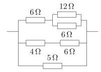
First calculate the resistance of the parallel  $12\,\Omega$  and  $6\,\Omega$  resistors in the top branch:
