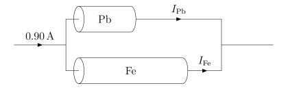
We can immediately see that both  $I_{\rm Fe}$  and  $I_{\rm Pb}$  will be less than  $I=0.90\,\rm A$ , and in fact  $I=I_{\rm Fe}+I_{\rm Pb}$ . The situation we have here is known as a *current divider*:
