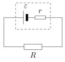
The diagram is a representation of a cell connected to a circuit of resistance R. The dashed box represents the outer case of the cell (within which we have no access), and the situation of internal resistance can be treated as though inside the battery there is an ideal cell (with no internal resistance) connected in series with a small resistor with
