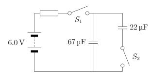
Initially, switch  $S_1$  is closed, charging the  $67\,\mu\text{F}$  capacitor from the battery.  $S_1$  is then opened, leaving the  $67\,\mu\text{F}$  capacitor fully charged and the  $22\,\mu\text{F}$  capacitor still uncharged. When switch  $S_2$  is closed, a spark occurs at the contacts of this switch. Estimate the energy dissipated in this spark. Is your value likely to be an over-estimate or an underestimate? Give a reason.
