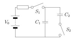
When  $S_1$  is closed, the capacitor  $C_1$  charges, to a charge  $Q = C_1V_0$ . The energy stored in  $C_1$  at this point is given by  $E = \frac{1}{2}CV^2 = \frac{1}{2}C_1V_0^2$ .
