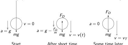
NB There is also a constant upward force of buoyancy, equal to the weight of
