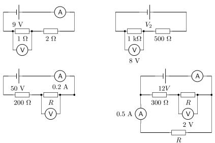
4. Calculate the resistance of the following networks of resistors.
