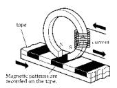
When someone is playing the tape, the magnetic patterns on the tape magnetize the ring, and this causes a current in the wire. The strength and direction of the current depends on the magnetic pattern on the tape. This electric current goes to a loudspeaker, which converts it into sound.
