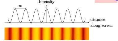
If the slit separation is s and the observation point is a distance D away (see diagram), then the width of the fringes w is given by
