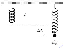
The way in which the length of a spring depends on the force on it was first investigated in the seventeenth century by Robert Hooke. He discovered that the extension of a spring from its natural length is directly proportional to the force applied to it and this is known as Hooke's law. Mathematically,
