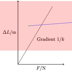
e.g. A typical spring which you might investigate in school will be stretched by about 5 cm by the weight of a 100 g mass. The weight force applied in this case is 1 N, and so the spring constant of such a spring would be  $20 \,\mathrm{N}\,\mathrm{m}^1$ . This could be checked by an experimental investigation measuring the extensions produced by different loads. The gradient of the graph of load against extension is the spring constant k (or the gradient of extension against load is 1/k).
